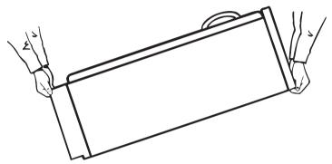
In order to push the appliance into its final position, press carefully at the top of the door and tip the appliance back slightly. The weight is then transferred to the back wheels and the appliance can be easily pushed.
